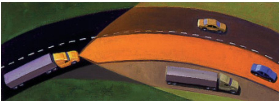
▲ Eaton® Vorad® EVT-300 detects hazards ahead even when the road curves left or right. Its patented monopulse technology, coupled with an internal yaw rate sensor, enables the system to distinguish between those vehicles ahead which present a danger and those vehicles in adjacent lanes which do not.
