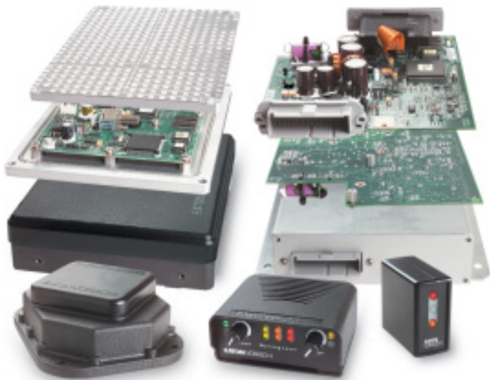
▲ Total weight of the Eaton® Vorad® EVT-300 Collision Warning System ranges from 4,5 kg with no side sensor to 6 kg with 2 side sensors.
